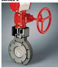
**Operation** Any residual air pressure in the pneumatic actuator must be vented before operation of the Declutchable Gear Operator. Bray recommends the use of a vent valve to block the incoming air supply and vent residual air. Then engage the declutching lever and rotate the valve using the handwheel. When returning to automatic operation, disengage the manual override by rotating the declutching lever, turning the vent valve to off, then restoring air pressure to the actuator.
